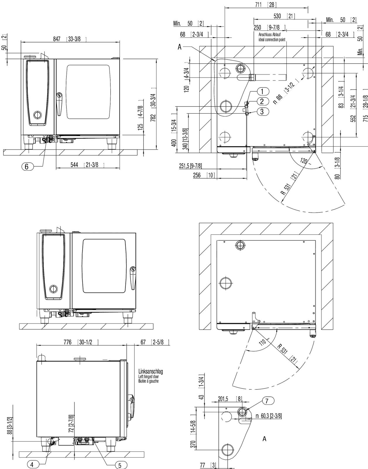
1. Common water supply (cold water) "Single" water connection as shipped
